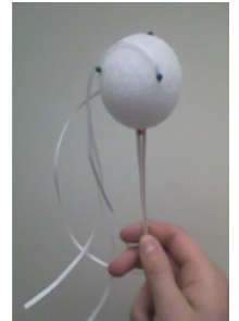
Figure 2. Paper streamers pinned onto foam ball
